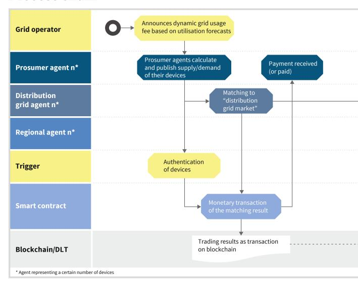
In this forward-looking use case, the distribution system operator dynamically adjusts the grid usage fee on the basis of current utilisation forecasting. Local electricity consumers and producers are thus incentivised to behave in a manner that is beneficial to the grid. In contrast to the use case "congestion management in electricity distribution grids (e-mobility)" (Use Case 1), market trading, which takes place here on a local market within
