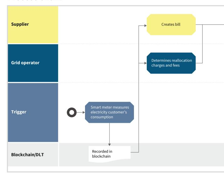
Processes in the energy industry, such as the billing of fees and reallocation charges, require data exchange between various market players. In this use case, a customer's consumption data is written to the blockchain via an intelligent metering system (smart meter gateway). An appropriate infrastructure is required
