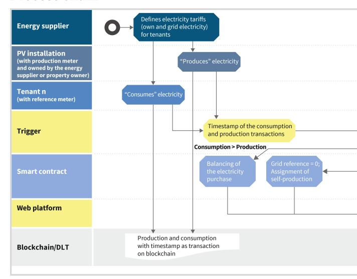
The aim of the blockchain-based interaction between the customer and owner of a landlord-to-tenant electricity supply property is to optimise local resources, i.e. the highest possible consumption of locally generated electricity. In the use case, the PV system is in the possession of the electricity supplier or the property owner, for instance. In addition to the electricity generation system, third-party tenants must also be considered in the
