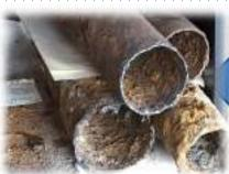
The heat supply system in Mytishchi had been built in the 1950-60s, and by the year 2000 the service period of heat supply facilities more 50 years, with more than 80% wear.
